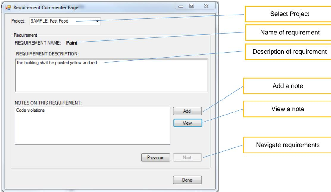
The dropdown at the top will allow the user to select any project the user has permissions to view. The "Next" and "Previous" buttons at the bottom will allow the user to view each requirement in sequence. The "View" button will allow the user to view the details of the note listed on its left. And the "Add" button will create a new note. The dialog presented to view/add a note is shown below.
